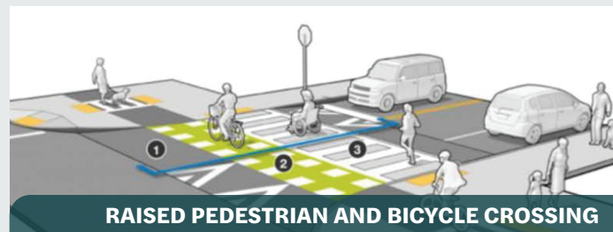
RAISED PEDESTRIAN CROSSING
